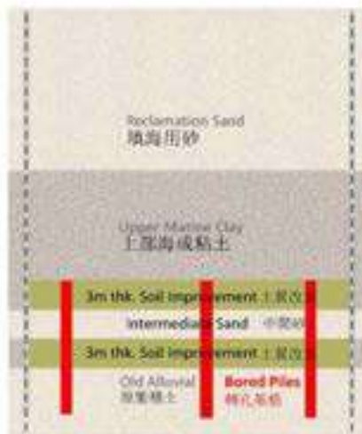
Installation of Foundation Bored Piles 安裝轉孔基樁
