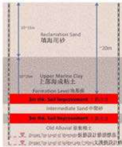
Soil Improvement works (injection of cement grout into the soil layer) 土質改良 (往土裏注入水泥漿)
