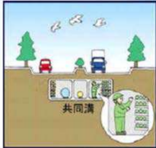
Fig. Accommodations in Common duct
